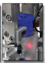
The CPC Capper can use a vibratory bowl, elevator, turntable, or gravity track to unscramble, sort and feed closures to the cap application station. A pneumatic container gating assembly is used to feed and securely clamp containers in place.
