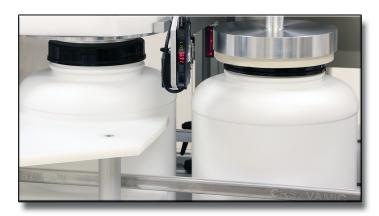
The Magna Capper uses a unique sorting elevator to hold, unscramble, and feed caps to the cap application station. A heavy-duty bottle gating assembly feeds and clamps containers in place. Caps are applied in the cap application station, then released and fed to the cap torquing station. There, the containers are clamped and a consistent torque is applied to the caps.
