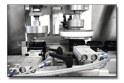
The Prime Capper uses a vibratory bowl to unscramble, sort and feed caps to the cap application station (optional sorting elevator available for larger caps). A pneumatic bottle gating assembly is mounted to any conveyor to index and clamp containers in place. Caps are applied in the cap application station, then released and indexed to the cap torquing station. Containers are clamped and consistent torque is applied.
