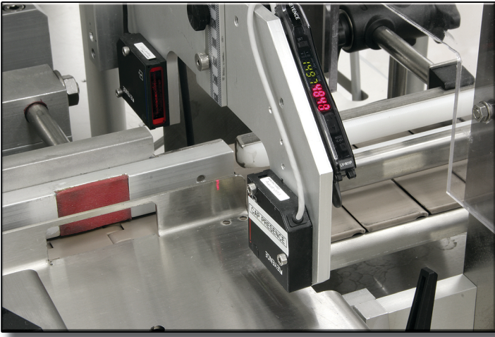
Plug/Tip Inspection Station
