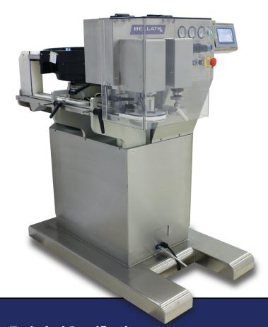
The Secure Chuck Capper uses a vibratory bowl to unscramble, sort and feed caps to the cap application station. A pneumatic bottle gating assembly is mounted to any conveyor to feed and clamp containers in place. Caps will be applied in the cap application station, then released and fed to the cap torquing station, where the containers are clamped and torqued consistently.
