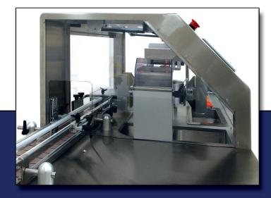
handles a wide range of containers. Quick setup features have been designed into the machine resulting in a machine that changes over in minutes. Mounted on casters, it can easily be wheeled to a convenient location in your plant where the recovery operation is to take place.
