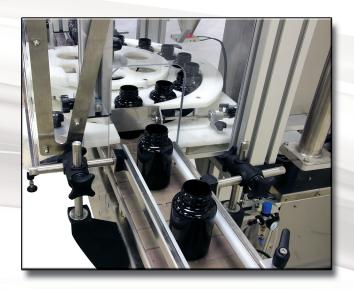
Scaled settings make repeat set ups fast and simple. Containers then need only satisfy the machine's start sensor and Rx-Desiccant PLUS will automatically index and insert desiccants into containers.
