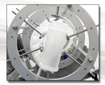
The Bell-Sort 100 is equipped with a sensor to detect and reject inverted bottles in the starwheel pockets. A slip clutch (torque limiter) protects the entire drive system from motor to starwheel.
