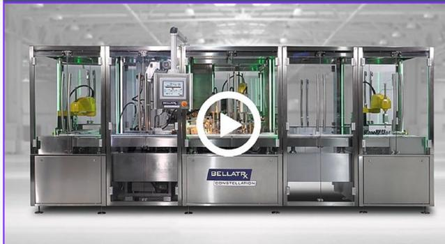
Some industries require extremely precise filling capabilities. BellatRx Constellation Monobloc uses unique liquid-filling technology to properly fill vials and tubes. Ideal for unstable microtubes, vials, and cartridges, the Constellation Monobloc uses **robotic pick and place stations** to unload vials from trays and reload the finished product back into trays.
